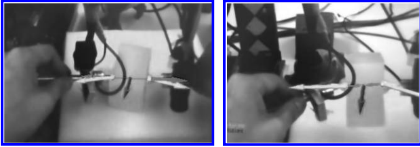
FIGURE 10.7 Example snapshot of visuo-haptic augmentation. Reaction force (dark gray arrow), weight (gray arrow), and haptic device force (light gray arrow) are depicted. Examples with increased stiffness (virtual forces oppose squeezing) and decreased stiffness (virtual forces assist squeezing) are shown on left and right, respectively.
